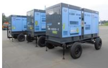
Fitting engine generators with wheels (Kashiwazaki-Kariwa)
