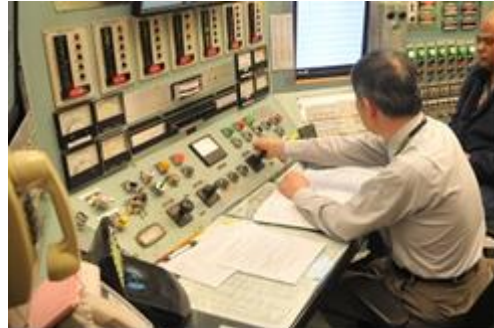
Operations and condition determination using a reactor simulator
