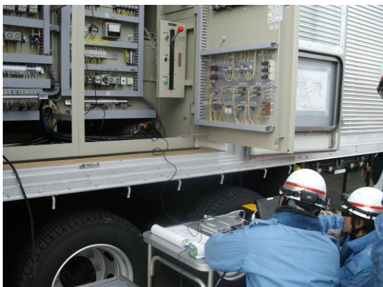
Failure diagnosis training for gas turbine power generator at Kashiwazaki Kariwa (Left: Confirming sequence logic of control car, Right: Confirming control parameters of gas turbine car)
