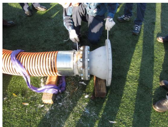
Temporary hose (Kanaflex) connection drill at Fukushima Daiichi (Left: Hose to hose connection, Right: Connection to different diameter flange)
