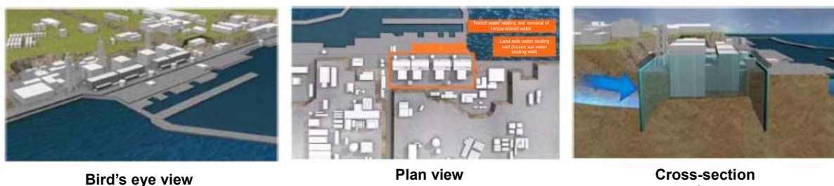
Overview of land-side water sealing wall work
