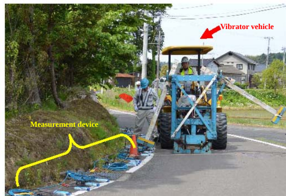
Subsurface prospecting in the vicinity of the plant site (Itsukaichi District)
