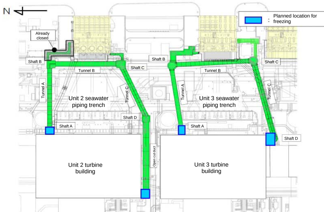
Layout of seawater piping trench
