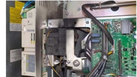
Soot inside the main winding inverter (May 11)
