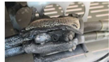
Damage of the inside of the brake register (May 12)
