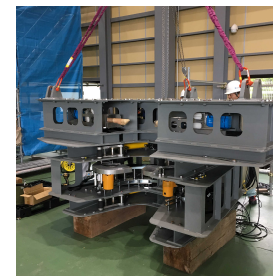
Steel tower disassembling device (for the main pillar)
