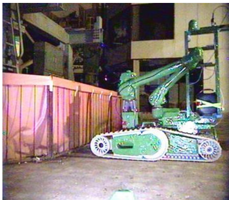
Using remotely operated robot to measure radiation levels
