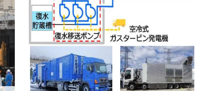
Substitute circulation cooling system
