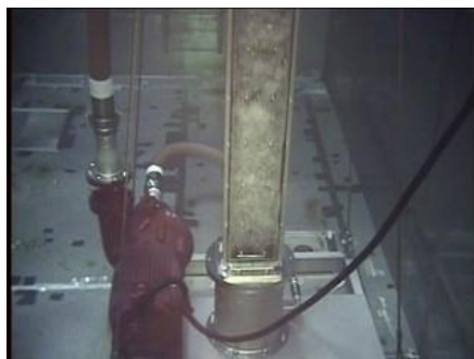
Fuel cleaning using air bubbles
