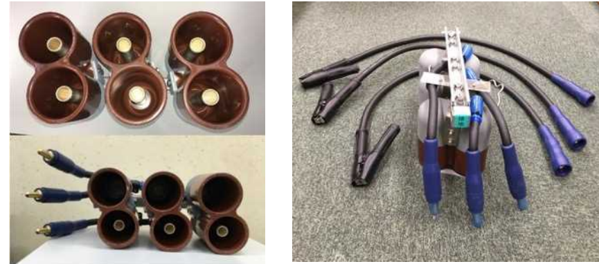
Top: Currently used tool (Closed-circuit kit) Full view of modified tool (earthing kit)
